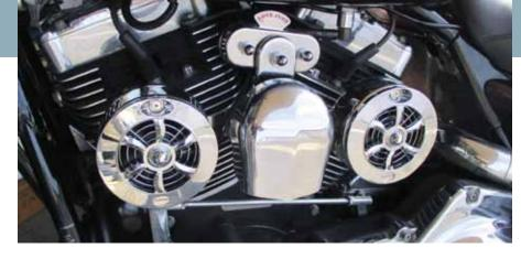
vided. The installation, including wiring and installing a switch, may take an hour or two, depending on the bike and the installer's skills. The Frame Mount Kit (for 2009 and newer models) requires gas tank removal and will take longer. For those mechanically-challenged folks, a Harley dealer or independent motorcycle shop should be able to do the job.
