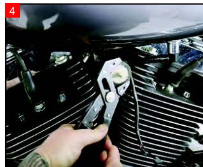
4 Use Vise-Grips or Channel-Lock pliers to remove the stock vibration isolator from the top motor bracket. This is usually difficult due to the thread locker used at the factory. It is okay if you destroy it during removal, it will not be reused.
