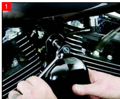
1 Use a 1/2" deep well socket to remove the acorn nut holding the horn bracket to the vibration isolator.
