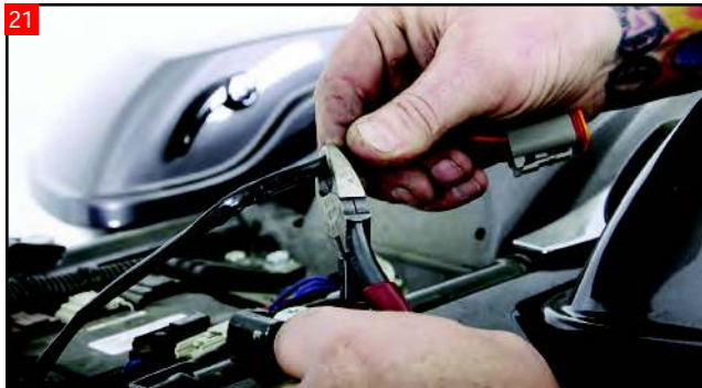
21 We elected to connect the Cool Master directly to the battery of the 2014 Street Glide. To do so, cut the accessory port plug from the Love Jugs' wiring harness.
