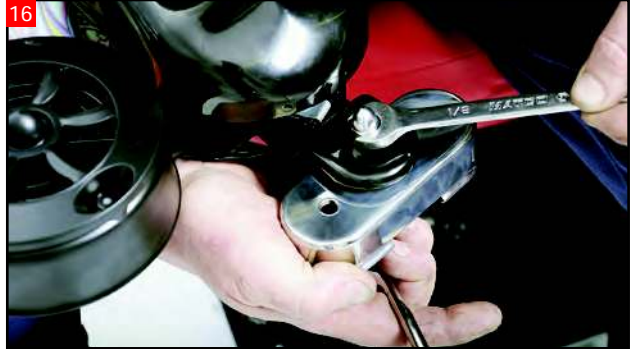
16 Install the polished cover, bracket and hardware on the stock horn bracket. Use the included acorn nut and washer to tighten.
