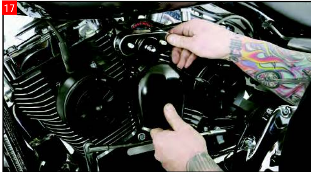
17 Position the Cool Master assembly over the two vibration isolators previously installed on the top motor bracket.
