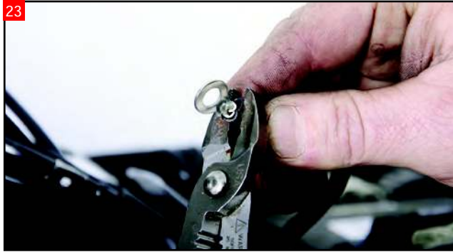
23 Crimp the black terminal to the negative wire.
