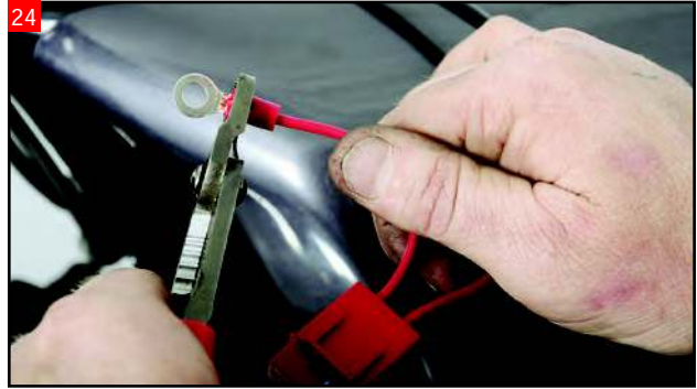
24 Install the in-line fuse to the positive (red) wire, and crimp the red terminal to the wiring from the fuse.
