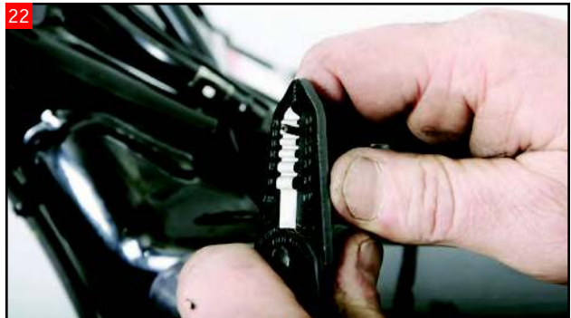
22 Strip 1/4" of insulation from the positive and negative wires.
