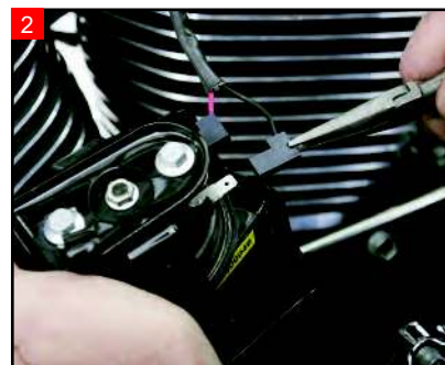
2 When removing the horn bracket from the isolator, turn it over to unplug the positive and negative wires for the horn.
