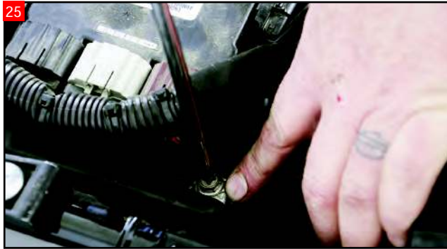
25 Install the red terminal to the positive of the battery and the black to the negative side.
