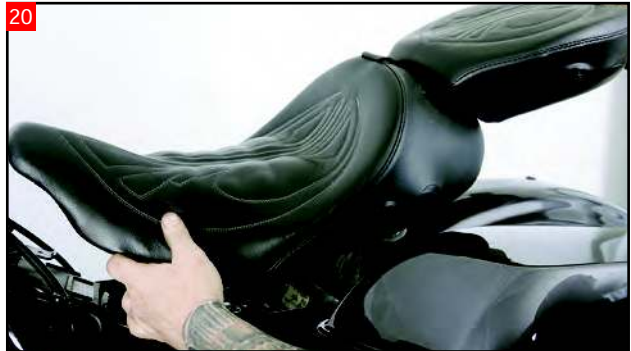
20 Remove the seat to access the battery. Carefully route the wiring from the Love Jugs to the battery compartment. Ensure the wiring is clear of any components that could get hot and burn a wire.
