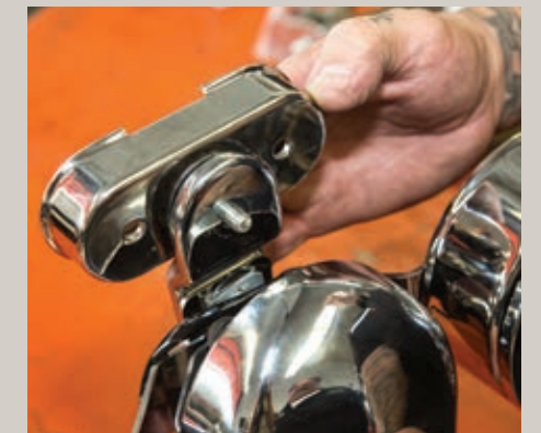
The Vibration Master's outer plate and the Cool Master fan assembly with the stock horn attached were bolted together.
