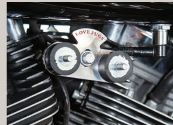
The Vibration Master was bolted to the factory horn-mounting bracket.
