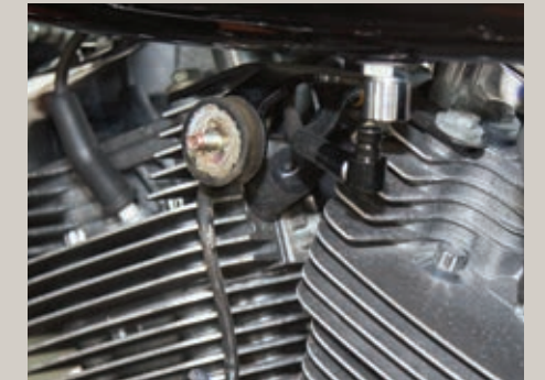
The Vibration Master will be attached to the factory horn-mounting bracket, which is bolted to the motor's cylinder heads.
