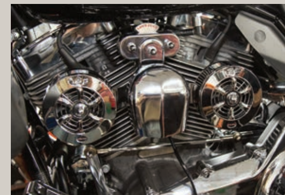
The completed fan assembly was bolted to the outer studs on the rubber isolators.
