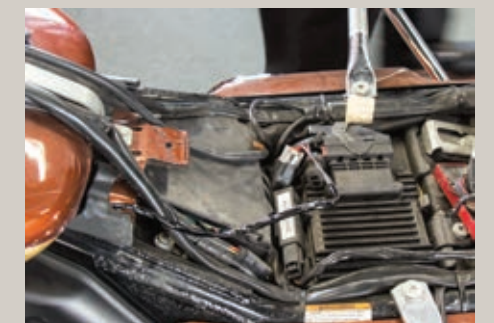
The Cool Master's wire harness was run back under the seat to the stock accessory harness connector and plugged in. The Love Jugs are now controlled through the accessory switch on the top of the fork cover.
