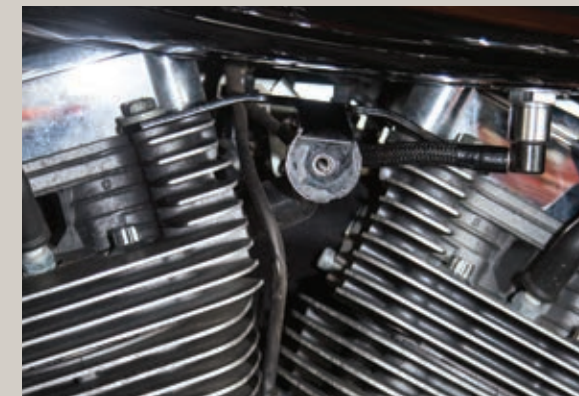
The factory rubber horn-isolating mount was unscrewed from its mounting bracket.
