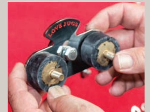
The Vibration Master's mounting plate uses two rubber isolators to support the Cool Master and the horn.
